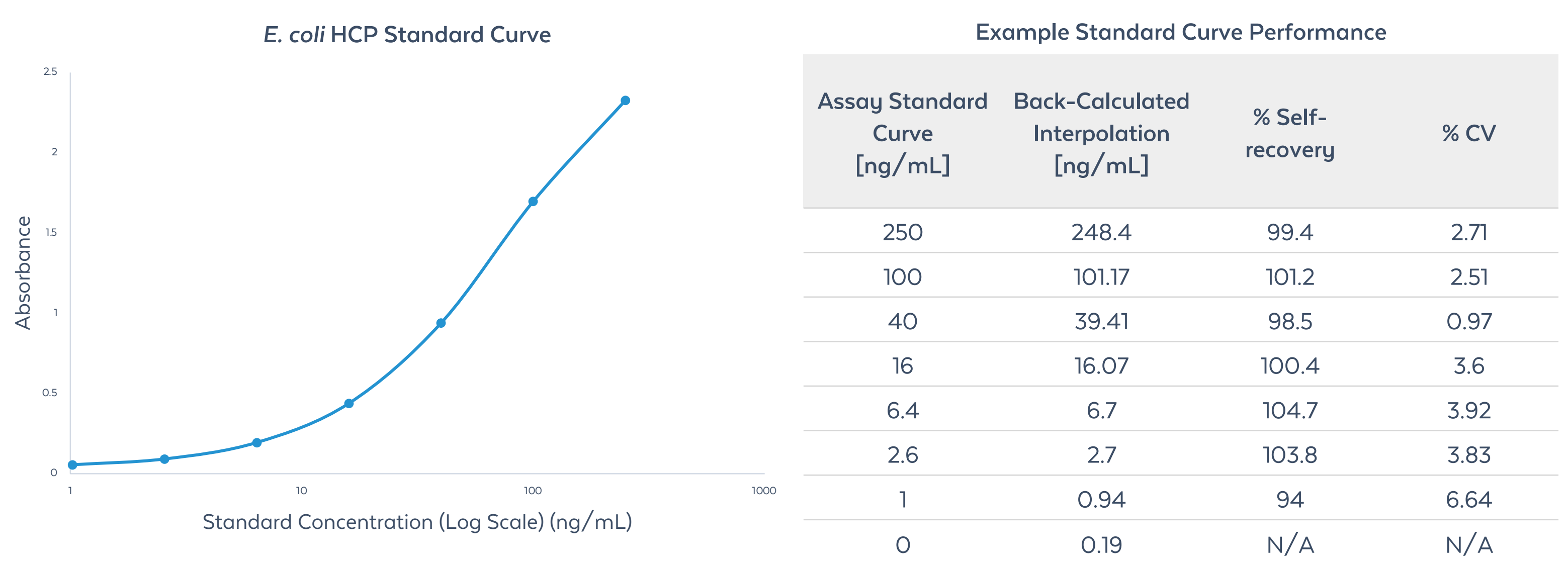
Figure 2. In developing this assay from the Rockland generated anti- E. coli HCP antibody, a standard curve needed to be created that: • Could successfully measure a broad range E. coli HCP concentrations • Had a high degree of accuracy as measured by its ability to back-calculate on itself (% Recovery) using a 4-Parameter Logistic Fit (L) • Had a high degree of precision as measured by the Percent Coefficient of Variance (% CV) of its replicates • Could be made in a series of user-friendly dilution steps After the rigorous testing of multiple options for standard curves, a dilution series was identified with a range of 1.0 - 250 ng/mL, with each standard curve point a 2.5x concentration dilution from the previous one. As a part of the initial assay development, optimal timing of capture, detection, and TMB development steps were identified, which demonstrated that this assay could successfully generate accurate and precise results in less than two hours.
